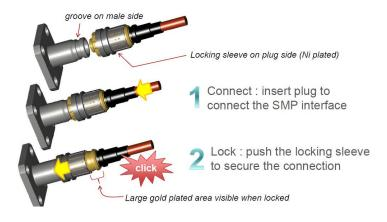
Fig1: Mating sequence of SMP-LOCK connectors
